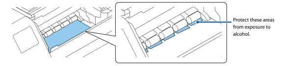
**7** Use a cotton swab or non-woven fabric moistened with alcohol to clean the roller. Carefully remove any labels that become stuck on the roller. Otherwise, they could cause a paper jam.
