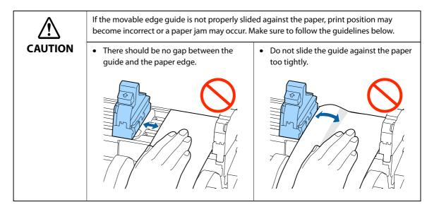
8 Insert the paper into the paper feed slot until paper feeding starts automatically.
