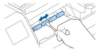
Rotating the roller using a cotton swab or non-woven fabric, remove the adhered paper dust or adhesive from the entire surface of the roller.
