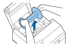
**1 1** Raise the paper guide unit, and then remove any jammed paper from the inside.
