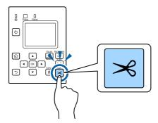
Press the [Back Feed] button to feed the paper backward.
