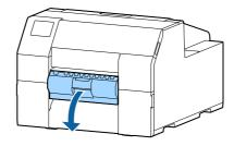
Cut the paper near the paper ejection slot.
