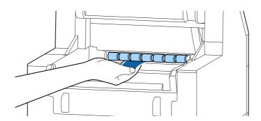
Rotating the roller by hand, remove paper dust or adhesive from entire surface of the roller.
