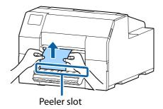
Hold down the Feed button until the paper is completely ejected.
