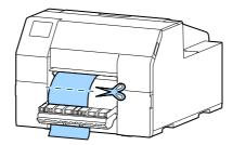
Press the [Back Feed] button to feed the paper backward.
