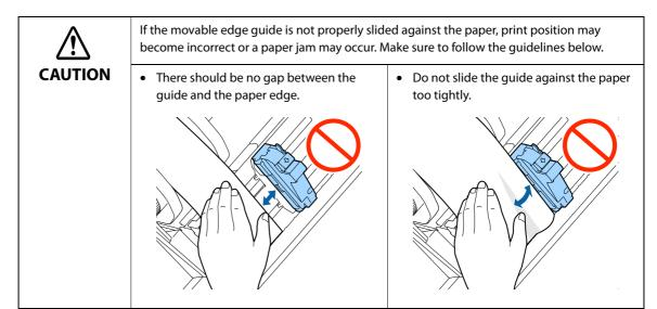
Insert the paper into the paper feed slot until paper feeding starts automatically.
