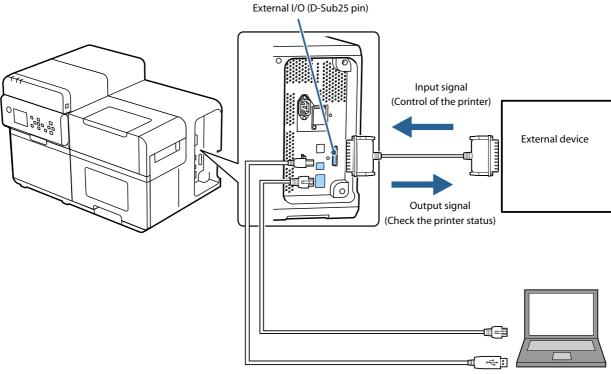
USB or Ethernet (Used to transmit commands)
