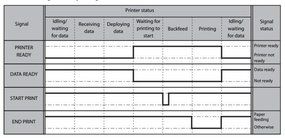
The pin 18 end print signal indicates that Mode 1 is set (= the printer feeds paper when Low).
