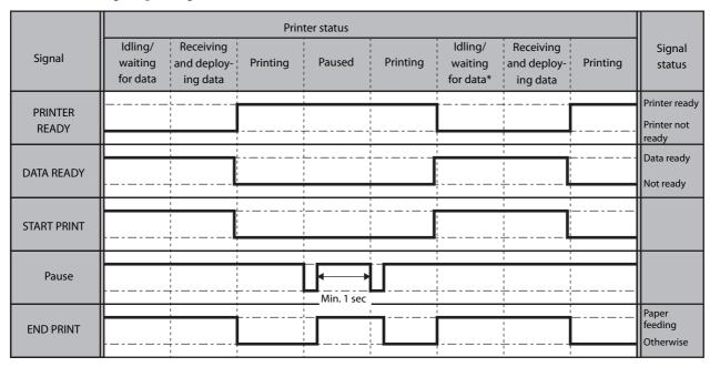
\* Once 1 second has elapsed to wait for data, the head is capped. When the head is capped, it takes about 2 seconds to start printing after the start print signal is given for the next print job.
