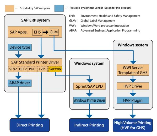
The **SAP Standard Printer Driver** used for Direct printing supports the following printer control languages.
