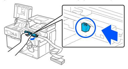
Raise the pressure unit with your finger placed on the tab (shown inside the circle below) and confirm that no labels is stuck to the pressure unit.
