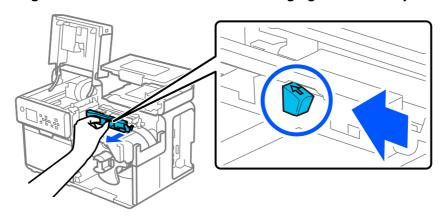
Raise the pressure unit with your finger placed on the tab (shown inside the circle below) and confirm that no labels is stuck to the pressure unit.
