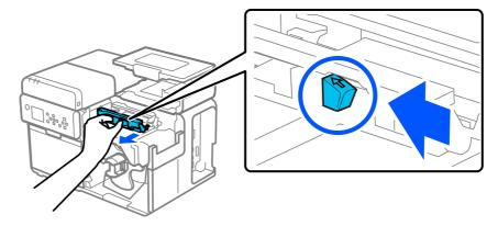
Remove labels, paper dust, and adhesive materials from the edge guides with a soft cloth dampened with water and wrung tightly.
