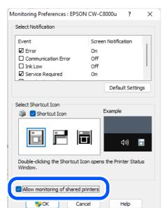
Select the check box for [Allow monitoring of shared printers], and then click [OK].
