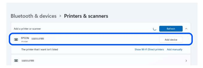
3 Wait until installation of the printer driver is finished.
