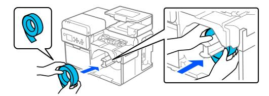
Attach the roll paper flange to the spindle while squeezing the levers of the flange. Move the flange until it touches the roll paper so that there is no gap in between.
