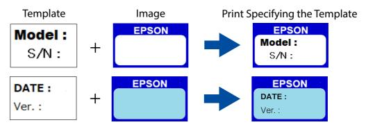
First store the image and the template data in the printer, and then make the link setting.
