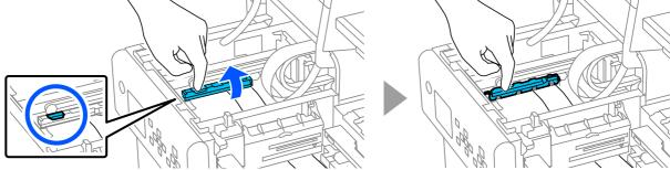
Raise the paper feed slot cover with your finger placed on the tab (shown inside the circle below) and confirm that no labels is stuck to the paper feed slot cover.
