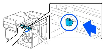
**10** Place the paper in the paper path along the edge guide and align the leading edge with the  $\sqrt{\phantom{a}}$  mark.
