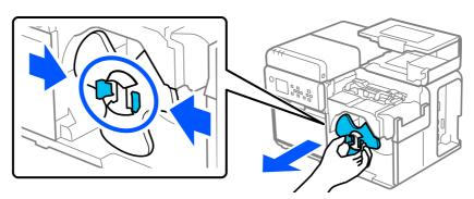
Attach a paper roll to the spindle and push the roll as far as it goes by pressing its core.
