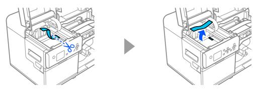
10 Wind up the paper by turning the roll paper flange clockwise until the leading edge of the paper passes through the paper feed slot.
