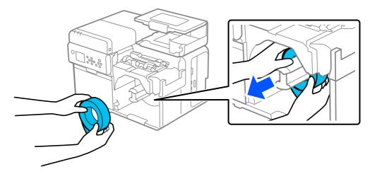
6 Attach the roll paper flange to the spindle.
