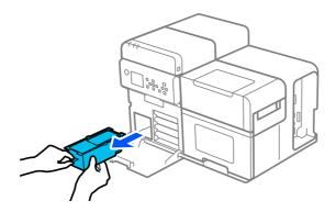
Seal the used maintenance box in a clear bag and dispose of it.
