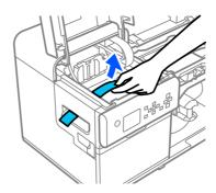
Manually cut the paper near the paper pressure rollers and remove it.
