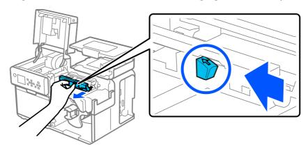
**7** Raise the paper feed slot cover with your finger placed on the tab (shown inside the circle below).
