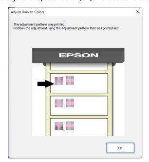
Enter the number for the most aligned group of horizontal lines and vertical lines in [Vertical direction] and [Horizontal direction], respectively, and click [Apply settings].
