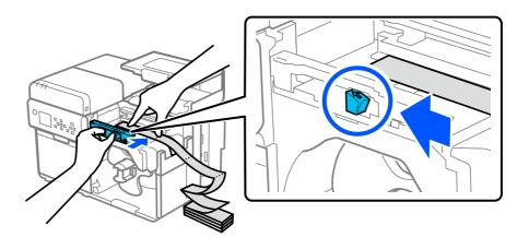
Insert the leading edge of the paper into the slot until the paper is automatically fed into the printer.
