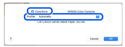
The default profile setting is [Automatic] which automatically selects an ICC profile provided by Epson. Select [Other Profiles...] to display the ColorSync profile selection screen and select a target ICC profile by yourself.
