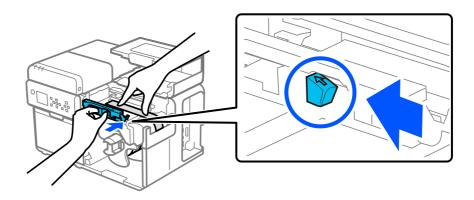
12 Insert the leading edge of the paper into the slot until the paper is automatically fed into the printer.
