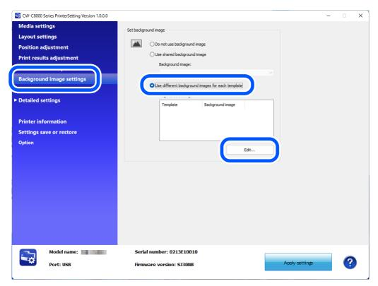
In the [Use different background images for each template] window, select a template and an image to be linked to the template, and then click [OK]. The link setting is set to the printer.
