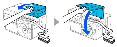
1 Place the stack of fanfold paper at least 15 mm {0.59 in.} away from the printer. Be sure that the paper is fed in a straight line to the paper feed slot.
