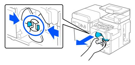
Remove the roll paper from the spindle.
