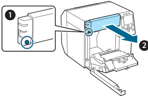
5. Disconnect the connector of the auto cutter unit from the printer.
