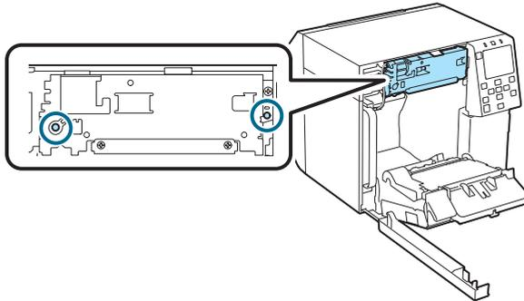
**9. Connect the connector of the auto cutter unit to the printer, paying attention to its orientation.**
