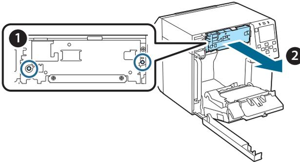
7. Install the replacement auto cutter unit. Align the holes on the left and right sides of the cutter unit with the protrusions on the printer. Otherwise, the unit may not operate properly.
