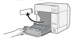
2 If the paper feed guide for fanfold paper is attached into the grooves inside of the roll paper cover, remove it.
