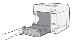
Remove the attachment for wristband.
