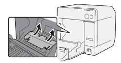
Install the attachment for wristband by inserting it into the grooves inside of the roll paper
