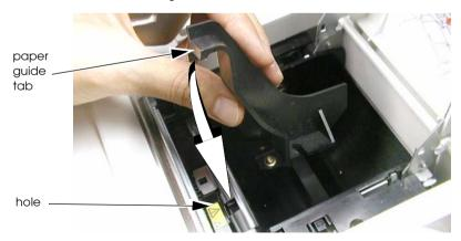
3. Slide the whole paper guide to the left for a 58 mm paper roll or to the right for a 60 mm paper roll as shown below. Be sure that the whole guide is in the correct position.
