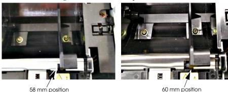
4. Insert and tighten the new screw provided with the paper guide.
