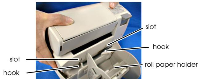
3. Attach the paper tray. Insert the hooks of the paper tray into the 2 slots in the bottom of the printer at the front. This completes installation of the roll paper unit.
