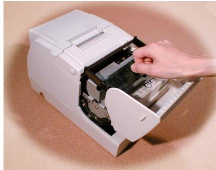
2. Turn the knob two or three times and check the ribbon position.
