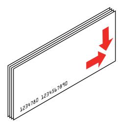
2 Insert documents straight with their faces (the side on which magnetic characters are printed) facing outside, as shown in the picture below.
