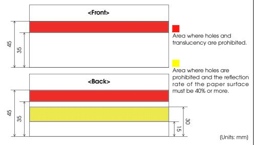
• The paper sensors ignore the range indicated in the figure below for the guide holes in fan-folded paper.
