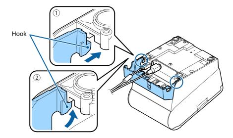
3. Push the connector cover down to click onto the printer case.
