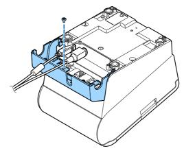
☐ To remove the connector cover, turn the printer over, remove the screw, and push the connector cover down while pushing both sides of the connector cover inward to detach the hooks from the printer case.
