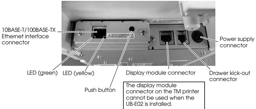
Note: This photograph shows the TM-H6000II printer with the UB-E02 installed.
