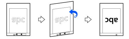
7. Load the Carrier Sheet into the input tray with the top edge facing into the ADF. Insert the paper into the ADF until it meets resistance.
