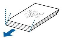
6. Load the originals with the side to be scanned facing down and the leading edge directed to the ADF. Insert the originals into the ADF until they meet resistance.
