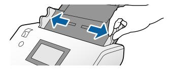
4. Load the originals at the center of the input tray in descending order of paper size with the widest at the back and the narrowest at the front.
