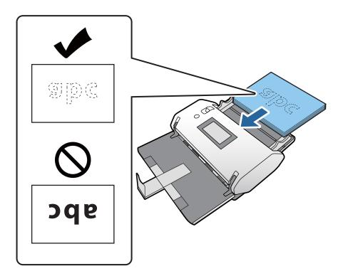
8. Adjust the edge guides to fit the original without any gap.
