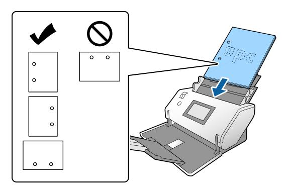
☐ If paper jams or double feeds frequently occur when scanning wrinkled paper, try to enable **Slow** to solve this problem. To do this, on the control panel, tap **Settings** > **Scanner Settings** > **Slow** and set it to **On** to slow down the feeding speed.
