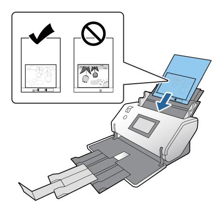
6. Align the edge guides with the Carrier Sheet without any gap.
