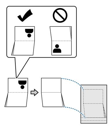
5. Load it into the input tray with the side to be scanned facing down and the side having a larger number of pages directed to the leading edge.
