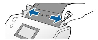
4. Load the original straight into the input tray with the side to be scanned facing down and its leading edge directed to the ADF.
