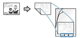
Load the Carrier Sheet with its leading edge directed to the ADF.
