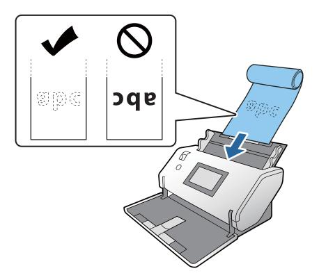
5. Adjust the edge guides to fit the original without any gap.
