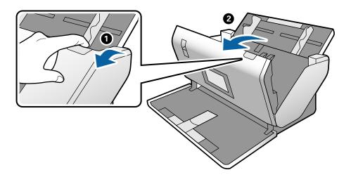
5. Wipe off any stains on the plastic roller and glass surface at the bottom inside of the scanner cover using a soft cloth or a genuine Epson cleaning kit.
