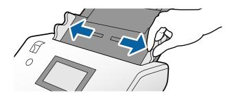
4. Load the envelopes longitudinally with the side to be scanned facing down into the input tray. For envelopes with an open end (flap portion) on the shorter side, load the envelope with the open end (flap side) placed at the top.
