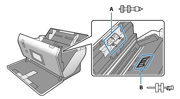
A: Separation Roller, B: Pickup Roller
