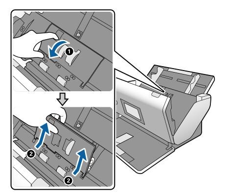
6. Pull down the fixture of the roller axis, and then slide and remove the installed Pickup Roller.
