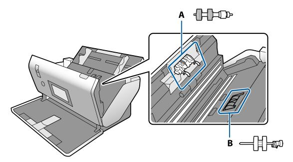
A: Separation Roller, B: Pickup Roller
