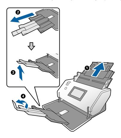
3. While holding the tab, slide the edge guides all the way out.
