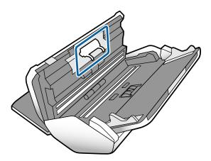
8. Wipe off any dust or dirt on the Separation Roller using a genuine Epson cleaning kit or a soft, moist cloth.
