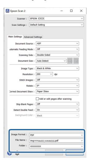
☐ **Image Format**: Select the file format for saving the scanned image from the list.
