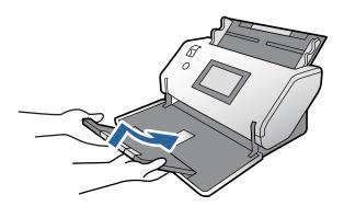
5. While keeping the position selector raised, slowly rotate the scanner to be in the Storage Position.
