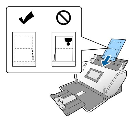
6. Align the edge guides with the Passport Carrier Sheet without any gap.
