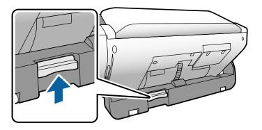
3. While keeping the position selector raised, slowly rotate the body of the scanner.
