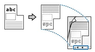
5. Load the Carrier Sheet with its leading edge directed to the ADF. Insert it into the ADF until it meets resistance.
