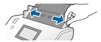
4. Load the cards with the side to be scanned facing down and their leading edge directed to the ADF. Insert the cards into the ADF until they meet resistance.
