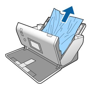
4. If you cannot pull originals straight up, carefully pull out any jammed originals from the output tray in the direction of the arrow.
