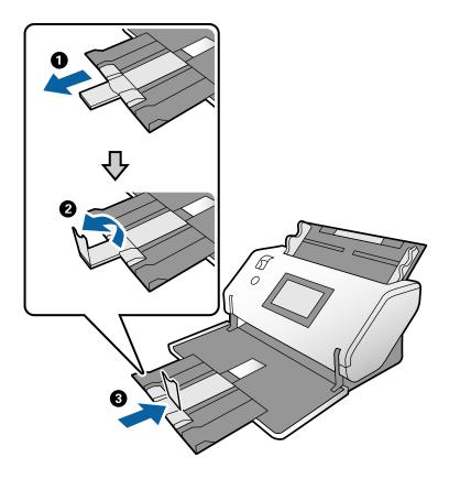
3. While holding the tab, slide the edge guides all the way out.
