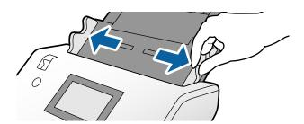
4. Load the passport with the thicker side aligned with the leading edge so that the side with the larger number of pages is pointing towards the leading edge.
