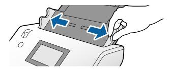
4. Load the booklet into the input tray with the printed surface facing down, and the thicker side pointing down, as shown in the diagram.
