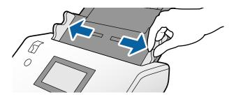
4. Make sure that the illustration at the edge of the Carrier Sheet is facing the front, and the original is facing the back when you insert the original into the Carrier Sheet.
