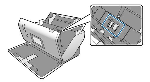
10. Wipe off any dust or dirt on the Pickup Roller using a genuine Epson cleaning kit or a soft, moist cloth.
