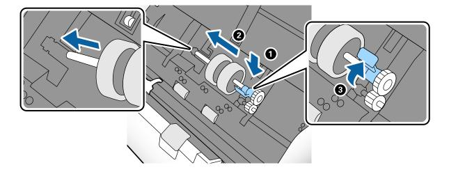
8. Put the edge of the cover of the Pickup Roller into the groove and slide it. Close the cover firmly.
