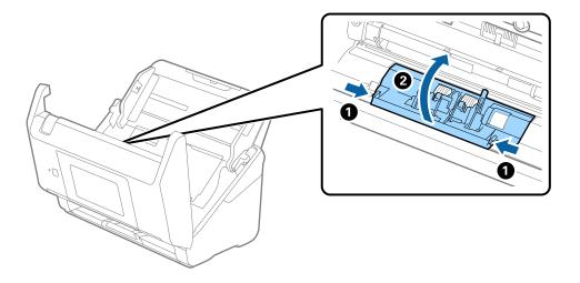
9. Lift the left side of the separation roller, and then slide and remove the installed separation rollers.
