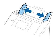
3. Load the laminated cards into the input tray facing down with the top edge facing into the ADF. Slide the laminated cards into the ADF until they meet resistance.
