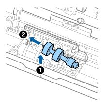
10. Insert the new separation roller axis into the hole on the right side, and then lower the roller.
