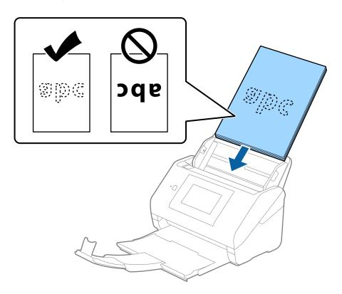
6. Slide the edge guides to fit the edge of the originals making sure there are no gaps between the originals and the edge guides. Otherwise, the originals may be fed skewed.
