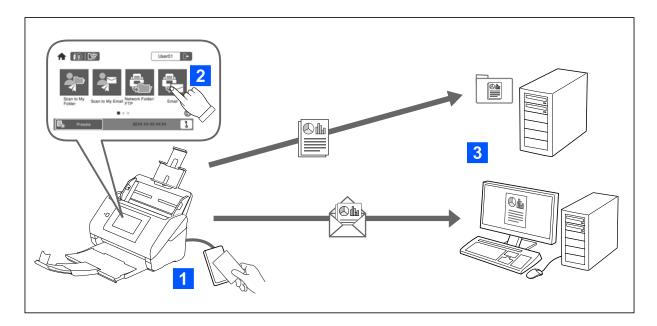
When the authentication setting is enabled on the scanner, user authentication is required to start scanning. You can set a different scanning method for each user, and prevent accidental operations.
