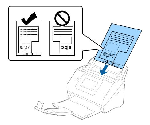
5. Slide the edge guides to fit the edge of the Carrier Sheet making sure there are no gaps between the Carrier Sheet and the edge guides. Otherwise, the carrier sheet may be fed skewed.
