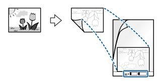
4. Load the Carrier Sheet into the input tray with the top edge facing into the ADF. Slide the Carrier Sheet into the ADF until it meets resistance.
