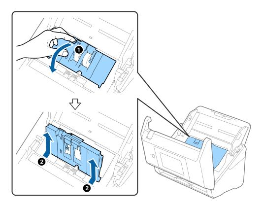
5. Pull down the fixture of the roller axis, and then slide and remove the installed pickup rollers.
