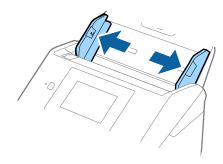
3. Load the original straight into the input tray, facing down with the top edge facing into the ADF. Slide the original into the ADF until it meets resistance.
