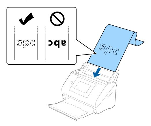
4. Adjust the edge guides to fit the edge of the long paper making sure there are no gaps between the edge of the paper and the edge guides. Otherwise, the originals may be fed skewed.
