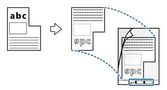
4. Load the Carrier Sheet into the input tray with the top edge facing into the ADF. Slide the Carrier Sheet into the ADF until it meets resistance.
