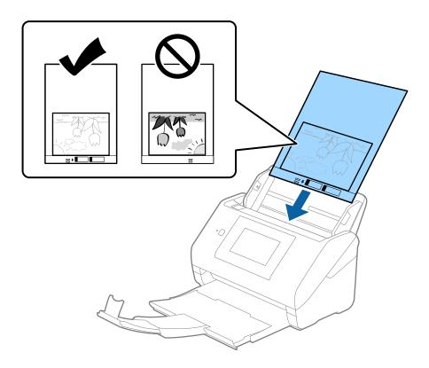
5. Slide the edge guides to fit the edge of the Carrier Sheet making sure there are no gaps between the Carrier Sheet and the edge guides. Otherwise, the carrier sheet may be fed skewed.
