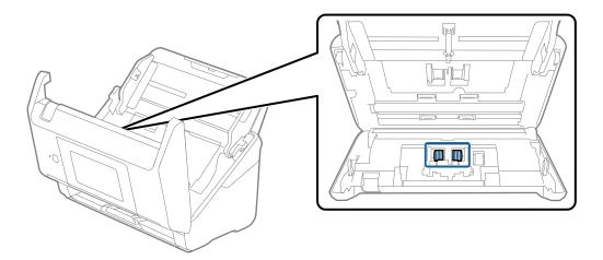
7. Wipe off any dust or dirt on the separation roller using a genuine Epson cleaning kit or a soft, moist cloth.
