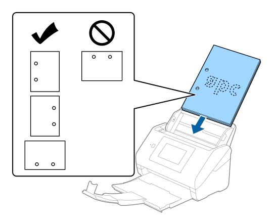
☐ When scanning thin paper with crinkles that are causing paper jams or double feeds, you may be able to improve the situation by enabling **Slow**. To do this, select **Settings** > **Scanner Settings** > **Slow** on the control panel and set it to **On** to slow down the feeding speed.
