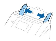
3. Place the Carrier Sheet with the illustration on the front edge facing up and place the original in the center of the Carrier Sheet with the side to be scanned facing down.
