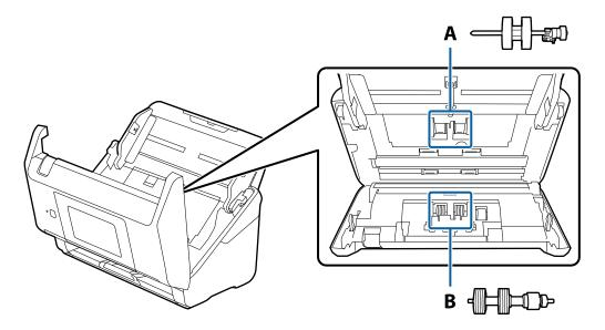
A: pickup roller, B: separation roller
