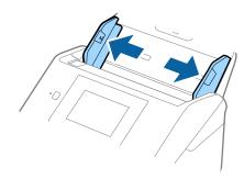
3. Place the Carrier Sheet with the illustration on the front edge facing up and place the photo in the center of the Carrier Sheet with the side to be scanned facing down.
