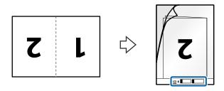
4. Load the Carrier Sheet into the input tray with the top edge facing into the ADF. Slide the Carrier Sheet into the ADF until it meets resistance.
