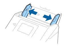
3. Load the envelopes into the input tray facing down making sure that the opened edge (flap side) of the envelope is facing to the side. For envelopes with the opened edge (flap side) on the shorter side, you can load the envelope with the opened edge (flap side) facing up.
