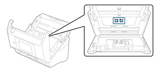
9. Wipe off any dust or dirt on the pickup roller using a genuine Epson cleaning kit or a soft, moist cloth.
