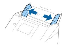
3. Load the originals at the center of the input tray in descending order of paper size with the widest at the back and the narrowest at the front.
