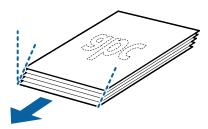
5. Load the originals into the input tray facing down with the top edge facing into the ADF. Slide the originals into the ADF until they meet resistance.
