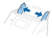
3. Load the plastic cards into the input tray facing down with the top edge facing into the ADF. Slide the plastic cards into the ADF until they meet resistance.
