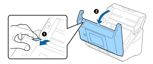
Open the cover of the pickup roller, and then slide and remove it.
