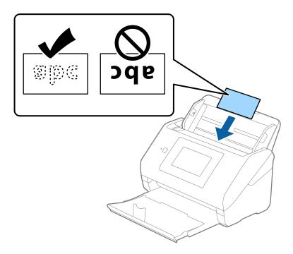
4. Slide the edge guides to fit the edge of the laminated cards.
