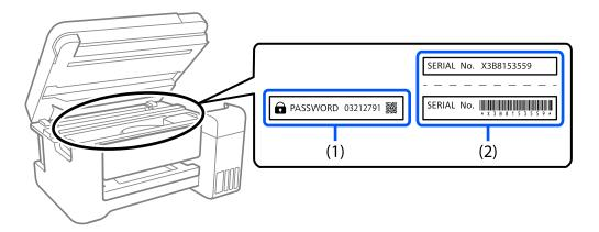
If both labels (1) and (2) are attached, the value next to PASSWORD written on the label in (1) is the default value. In this example, the default value is 03212791.
