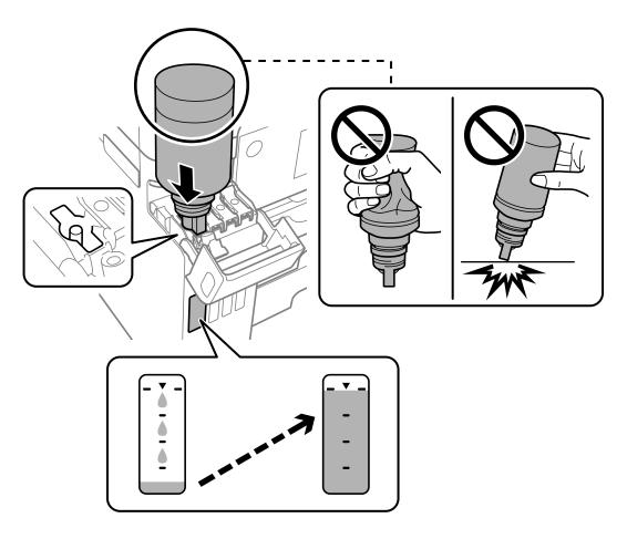
When you have finished refilling the ink, remove the ink bottle, and then close the ink tank cap securely.
