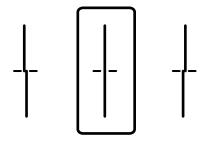
☐ This pattern allows you to perform alignment if you see horizontal banding at regular intervals. Find and enter the number for the least separated and overlapping pattern.
