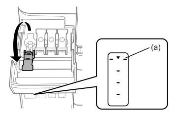
8. Align the top of the ink bottle with the filling port, and then insert it straight into the port to fill ink until it stops automatically at the upper line.
