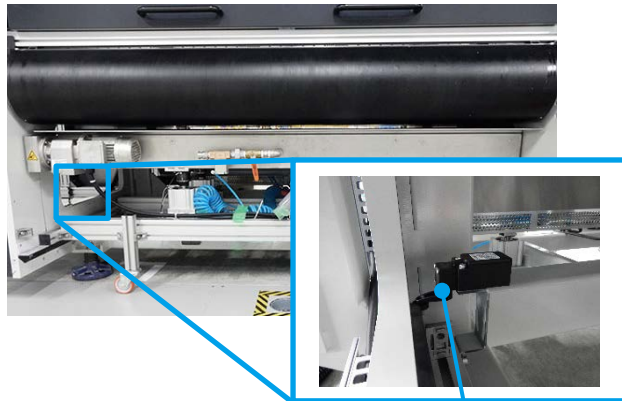
Belt cleaning unit position sensor
