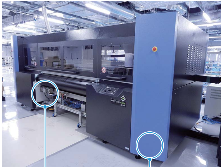
Waste ink tank on the flushing area side
