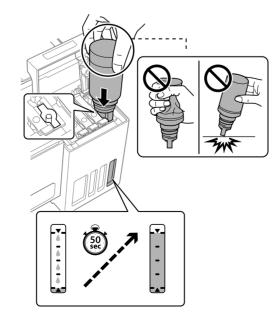
☐ When you insert the ink bottle into the filling port for the correct color, ink starts pouring and the flow stops automatically when the ink reaches the upper line.
