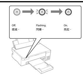
The nozzle check pattern is printed. Check the printed pattern to see if the print head nozzles are clogged. 將列印噴嘴檢查圖案。檢查列印的圖案以查看印字頭噴嘴是否
