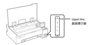
Insert the ink bottle straight into the port to fill ink to the upper line. 將墨水瓶徑直插入填充口以填充墨水至最高標示線。
