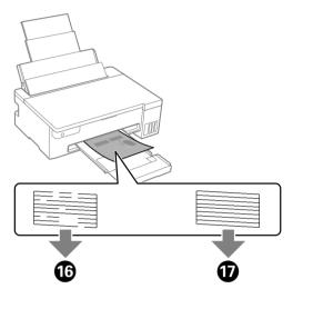
Run the print head cleaning. Print head cleaning uses some ink from all ink tanks.
