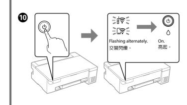
Confirm that the tanks are filled with ink, and then hold down the  $\odot$  button for 5 seconds to start charging ink. Charging ink takes about
