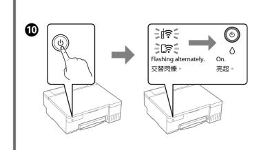
Confirm that the tanks are filled with ink, and then hold down the button for 5 seconds to start charging ink. Charging ink takes about
