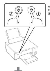
While holding down ①, press ② to turn on the printe 按住①時,按下②以開啟印表機。
