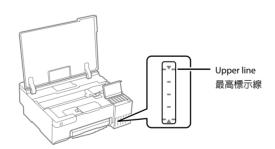
Insert the ink bottle straight into the port to fill ink to the upper line. 將墨水瓶徑直插入填充口以填充墨水至最高標示線
