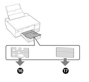
Run the print head cleaning. Print head cleaning uses some ink from all ink tanks. 執行印字頭清潔。清潔印字頭時,將使用所有大容量墨水槽中
