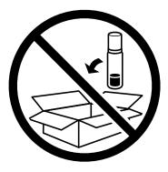
When you use the printer again, make sure you remove the tape securing the ink tank. If print quality has declined the next time you print, clean and align the print head.
