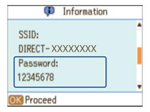
8. After the connection is established, press the OK button on the printer's control panel.
