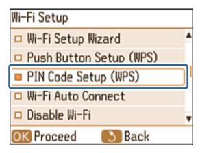
5. Use your computer to enter the PIN code (an eight digit number) displayed on the printer's control panel into the access point within two minutes.
