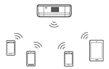
The printer can be connected by Wi-Fi and Simple AP mode simultaneously. However, if you start a network connection in Simple AP mode when the printer is connected by Wi-Fi, the Wi-Fi is temporarily disconnected.
