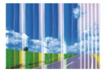
The print head nozzles may be clogged. Perform a nozzle check to check if the print head nozzles are clogged. Clean the print head if any of the print head nozzles are clogged.
