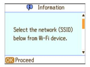
6. Check the SSID and password displayed on the printer's control panel. On the network connection screen of the smart device, select the SSID shown on the printer's control panel to connect.
