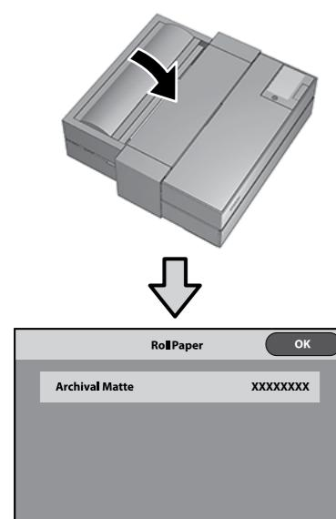
Close the roll paper cover and choose the paper type on the screen. Press [OK] to initiate the feed operation.
