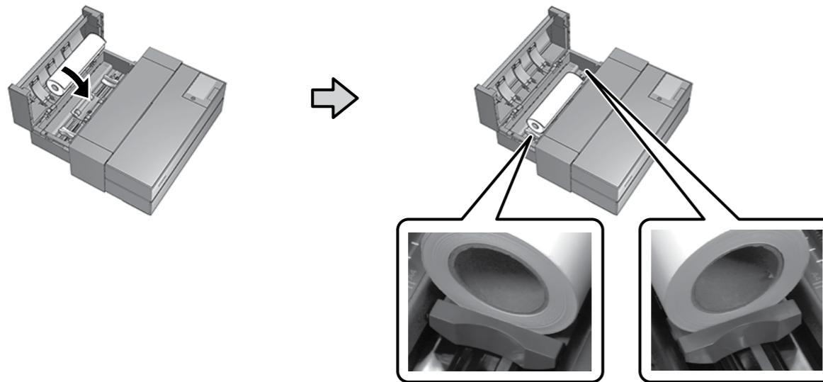
Load the roll. Check that the edge guides are positioned at the ends of the roll.
