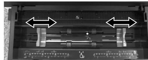
Position the edge guides to match the width of the roll.
