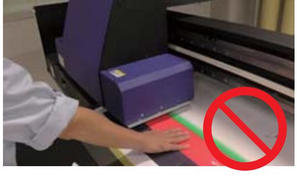
A photograph showing a person's hand reaching very close to the purple printer head, almost touching it. A large red circle with a diagonal slash is overlaid on the image to indicate it is incorrect.        |
