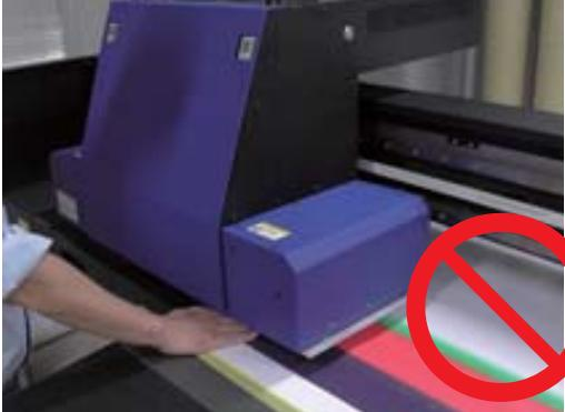
A photograph showing a person's hand reaching into the gap between the blue paper carriage and the support table. A large red circle with a diagonal slash is overlaid on the image to indicate it is incorrect. |
