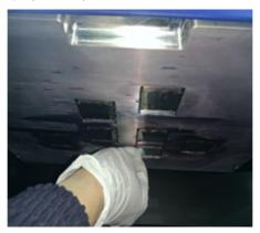
1-5 Apply the cleaning liquid to the polyester/nylon knit woven fabric, and then clean the UV lamps on both sides of the carriage. If the ink has hardened, use a scraper or a similar tool to remove it.
