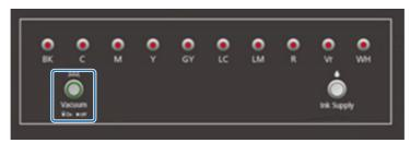
2-2 Open the valve according to the position in which the media is loaded. The media sticks to the table.
