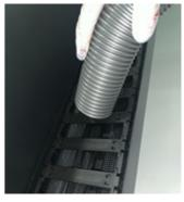
Use a vacuum cleaner and so on to suck up any dust that has accumulated on the filter for the UV lamp cooling unit.
