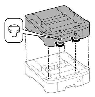
8. Lower the printer gently onto the optional paper cassette aligning the corners, and then secure them with the screws using the screw driver that came with the optional paper cassette unit.
