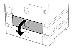
5. Remove the screws by a screwdriver and remove the cover on the rear of inside the printer.
