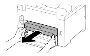
6. Remove the cover inside the back of the printer.
