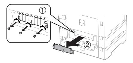
6. Slide out two used maintenance rollers, and remove both of them.
