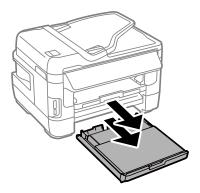
For WF-7610 Series/WF-7620 Series: Remove the cover.
