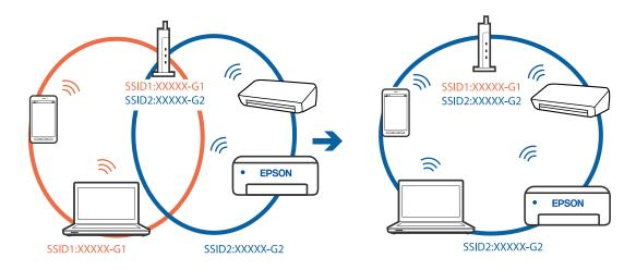
☐ Example of connecting to SSIDs with a different frequency range
