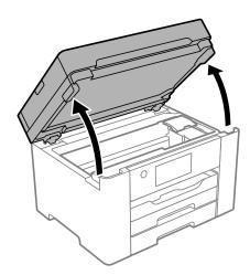
3. Check if the translucent film is smeared. Smears are easier to see if you use a light. If there are smears (such as finger marks or grease) on the translucent film (A), go to the next step.
