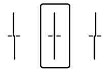
☐ This pattern allows you to perform alignment if you see horizontal banding at regular intervals. Find and select the number for the least separated and overlapping pattern.
