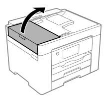
2. Use a soft, moist cloth to clean the roller and the interior of the ADF.
