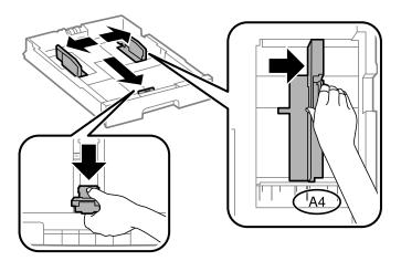
Load paper with the printable side facing down, and then slide the front edge guide to the edge of the paper.
