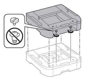
8. Lower the printer gently onto the optional paper cassette aligning the corners, and then secure them with the screws using a screw driver.
