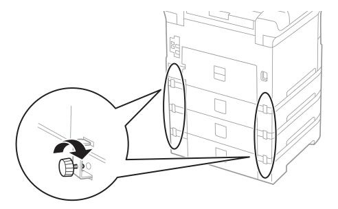
10. Insert a label showing the size of the paper to be loaded in the cassette into the holder.
