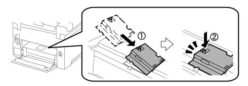
10. Hold up the maintenance roller for the paper cassette by rolling it up, and then remove it.
