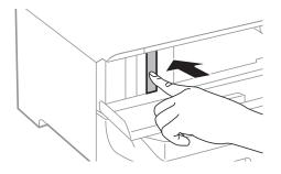
3. Remove the ink cartridge from the printer.
