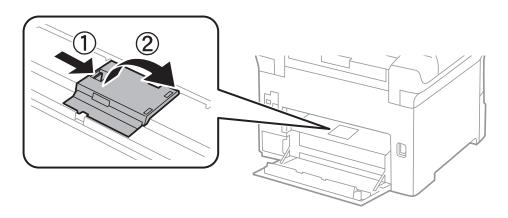
7. Slide out the two used maintenance rollers, and remove them.
