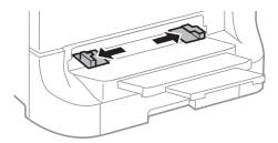
3. Insert the paper with the printable side facing down until the printer partially pulls in the paper.
