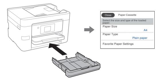
If displayed paper size and type differ from the loaded paper, select the item to change. If the settings match the loaded paper, close the screen.
