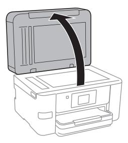
Use a soft, dry, clean cloth to clean the surface of the scanner glass.
