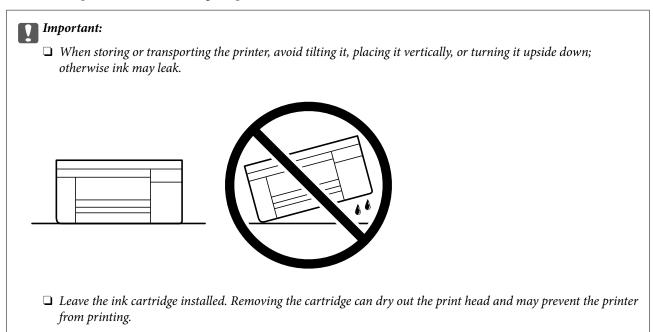
When you use the printer again, make sure you remove the tape securing the ink cartridge holder. If print quality has declined the next time you print, clean and align the print head.
