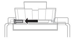
3. Load paper vertically along the right side of the rear paper feed with the printable side facing up.
