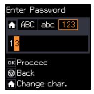
4. Press the ▶ button once to move the cursor, and then press the ♠ button to switch the character type to ABC. Press the ♠ button twice to select "B".
