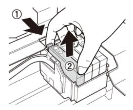
6. Insert the new ink cartridge, and then press it down firmly.
