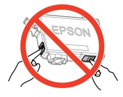
$oldsymbol{\square}$  Do not shake cartridges after opening the package, as they may leak.
