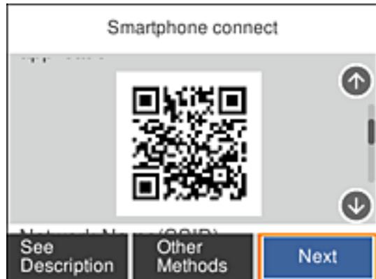
4. On your iPhone, iPad, or iPod touch, start the standard Camera app, and then scan the QR code displayed on the printer's control panel in PHOTO mode.
