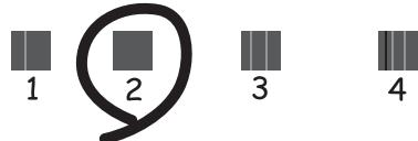
**Horizontal Alignment**: Find and select the number for the least separated and overlapping pattern.
