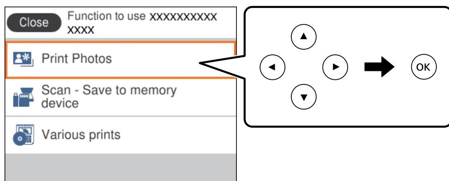
To select an item, move the focus to the item using the **▲** **▼** **◀** **▶** buttons, and then press the OK button.
