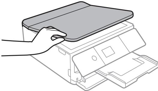
2. Remove any dust or stains on the surface of the scanner glass using a soft, dry, clean cloth.
