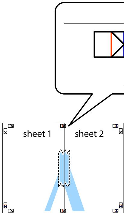
3. Cut the taped sheets in two along the vertical red line through the alignment markers (this time, the line to the left of the cross marks).
