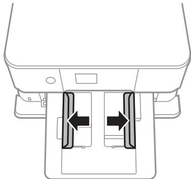
5. With the printable side facing down, load paper until it touches the back of paper cassette 1.
